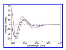
**Figure 5.** Experimental and calculated ECD spectra of 1 (black, experimentally observed in methanol; blue, calculated in the gas phase; red, calculated in methanol).
